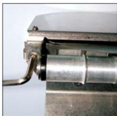
The cutting strength can be infinitely adjusted from 0mm to 6mm on the guide roll. Loosen the screws, set the cutting strength and tighten the screws again slightly for this. Meat slices and poultry meat are generally cut thicker than minced meat.
