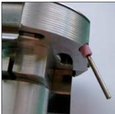
Depending on the operating time, the circular knife should be re-sharpened. This can be done without dismantling the knife. For this, start the unit and pull out the circular knife with the aid of the grinding pin by gently applying pressure and turning at the same time. Repeat this process from time to time. Never check the sharpness of the circular knife without unplugging the device from the power supply beforehand. **Danger of injury!**
