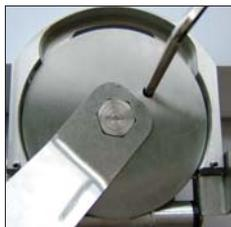
If the device is not used for longer periods, a more intensive cleaning is advisable. For this, unplug the device from the power supply as shown, dismantle the circular knife, loosen the knife head locking and remove the knife head. The device can now be cleaned. The device is assembled in the reverse order. Ensure that the knife head screw is not tightened too firmly and that the locking key is removed before operation!
