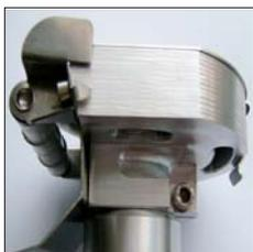
In order to turn the knife head radially on the handle piece, loosen the locking screw, turn the handle until it rests optimally in the hand of the user and now pull the locking screw tight again (max. 3Nm). Ensure that the knife head is pressed completely backwards in order to prevent the circular knife from grinding against the stripping plate.
